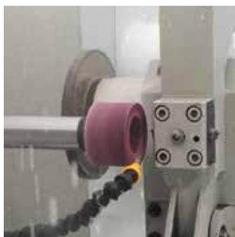
> Internal grinding wheel dresser with single point diamond.
